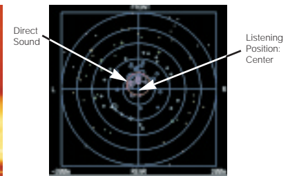
Virtual sound sources are blue or white rounds. Round scale is a reflection strength.
